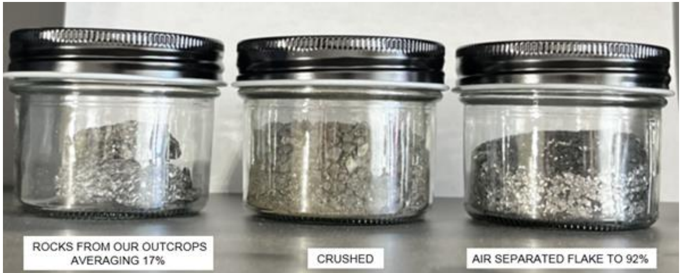
Figure 1: Samples of ore, feedstock and air separated graphite
